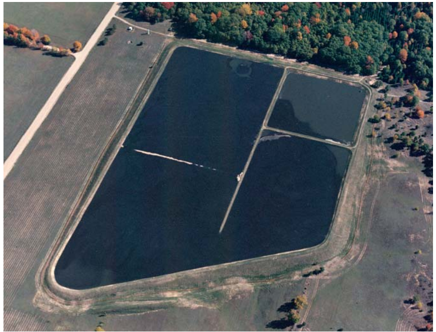
Figure 18. Dredged sediment disposal cell (aerial view).
